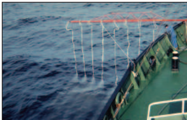
Boat application using spray arms mounted near the bow of the vessel.
