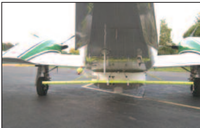
Spraying boom under a Cessna 406 (Photo courtesy of CEDRE).
