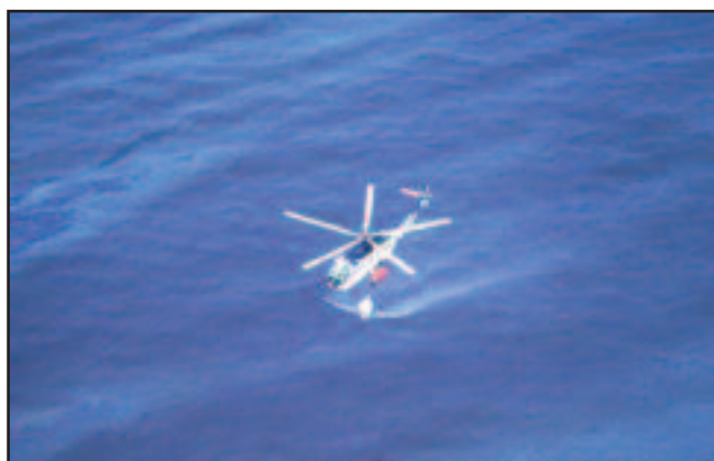
Aerial application of dispersant using a helicopter and underslung spray bucket system.
