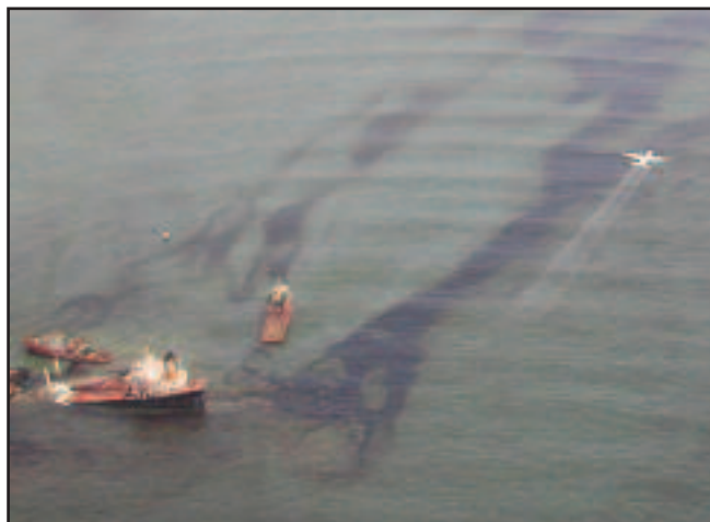
Aerial application of dispersant using an ADDS pack and Hercules aircraft.
