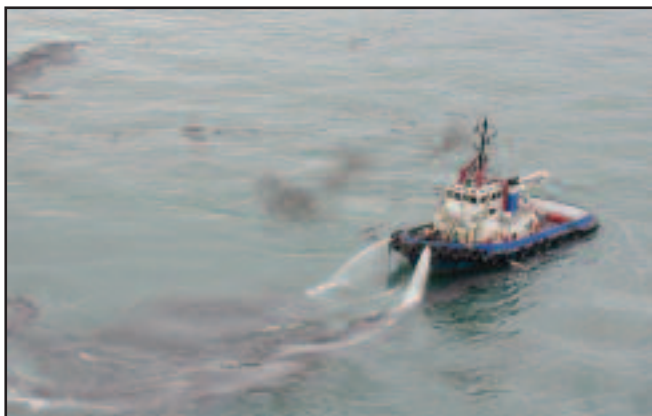
Unsuccessful application of dispersants on a non dispersible heavy oil using fire monitors on a tug.
