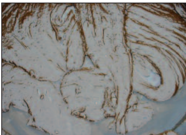
The dissipation of many oils is slowed by the formation of highly viscous water-in-oil emulsions.
