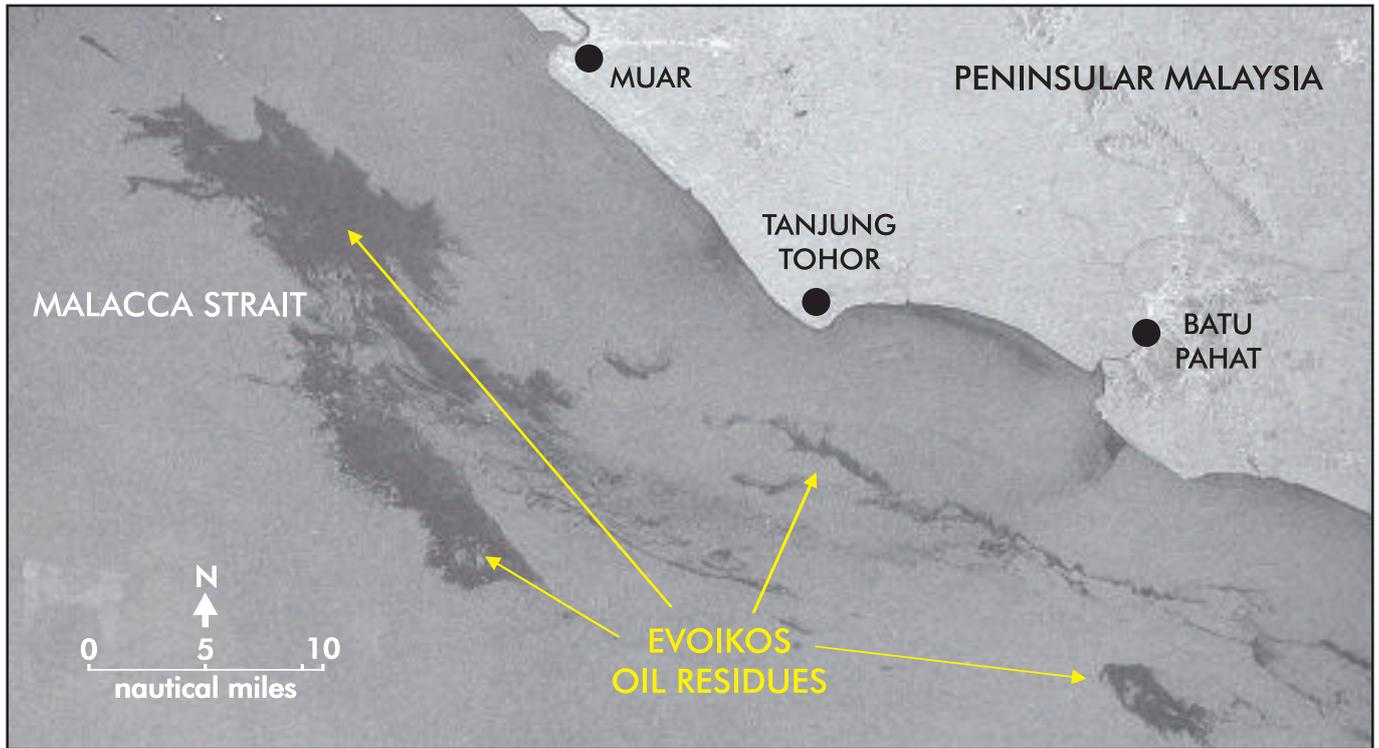
**Figure 18:** A Synthetic Aperture Radar satellite image of the southern Malacca Strait taken after the EVOIKOS spill in Singapore, showing the oil residues whilst they were moving north-west with the current. Image kindly provided by RADARSAT International © Canadian Space Agency 1997. Received and processed by CRISP, National University of Singapore and distributed under licence by RADARSAT International.
